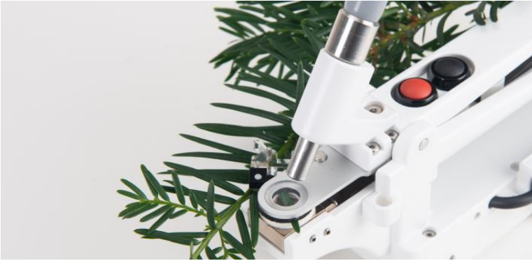
Fig. 7: Black gaskets for sealing specific samples.
