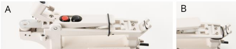
Fig. 3: Black ring holding the chamber in an open position (A) and tucked away for measurements (B)
