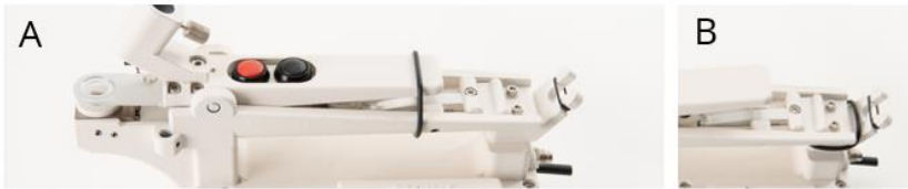
Fig. 10: Black ring holding the chamber in an open position (A) and tucked away for measurements (B)
