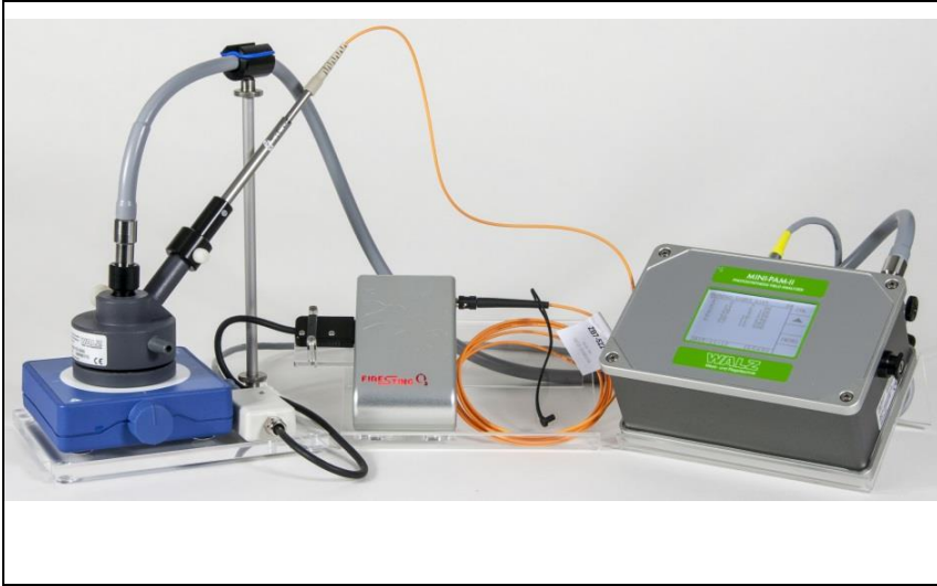
Fig. 24: O 2 measurement. System Overview
