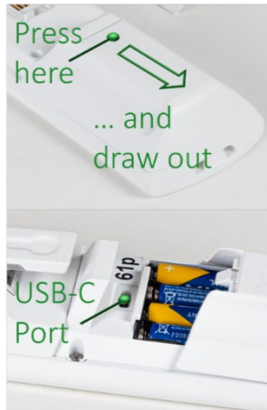
Fig. 9: Access to USB-C Port
