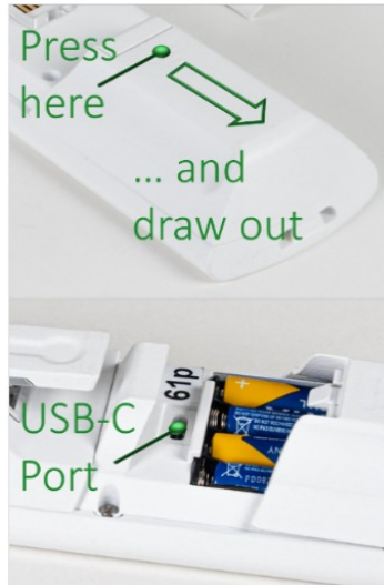
Fig. 12: Access to USB-C Port
