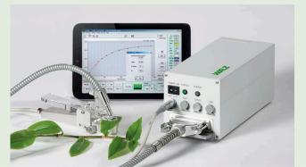
The PAM-2500 Portable Chlorophyll Fluorometer is the successor of the well-known PAM-2000/2100 instruments which were introduced in the 1990s as the first portable PAM fluorometers. Since then they have been successfully applied worldwide by numerous scientists. In the development of the PAM-2500, particular care was taken to maintain all properties appreciated by PAM-2000/2100 users and, at the same time, to integrate state-of-the-art technology.
