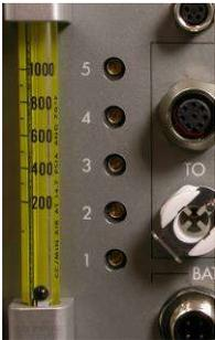
The adjustment of the internal restrictor valves (see Fig. 3) can be necessary after changing the flow rate or the measuring head of the GFS-3000. The valve adjustment tunes the system, so that the pressure in the reference and sample cell of the analyzer is equal. Also the total flow through the system or analyzer in MP mode and ZP is adjusted with the valves. The flow through the analyzer is shown by the mechanical flow indicators attached to the front panel (Fig. 2).
