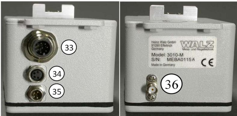
Fig. 10: Connectors at the rear side and front side of the electronics box
