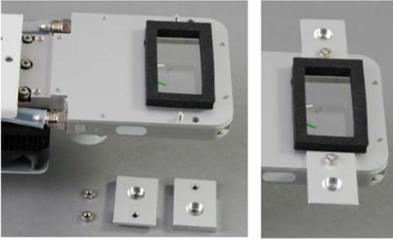
Attach the leaf area adapter plate to the cuvette frame, keep the blue O-ring in place. Use two long screws to attach the protruding plates. Connect the rear legs as shown in the first picture of this chapter.
