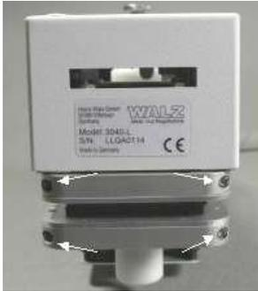
The light source, imaging-PAM or darkening plate can be mounted on either side of the Standard Measuring Head 3010-S by clicking its pins into the coupling of the respective cuvette frame. To tighten or loosen this connection, the screws on the front of the cuvette frames can be adjusted (*see picture*).
