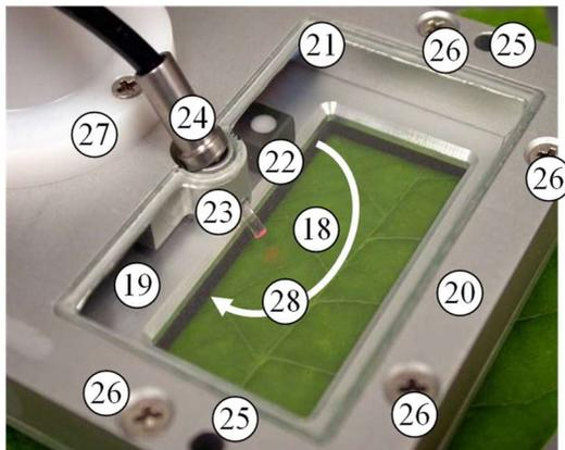
Fig. 8: View from the top onto the upper half of the cuvette
