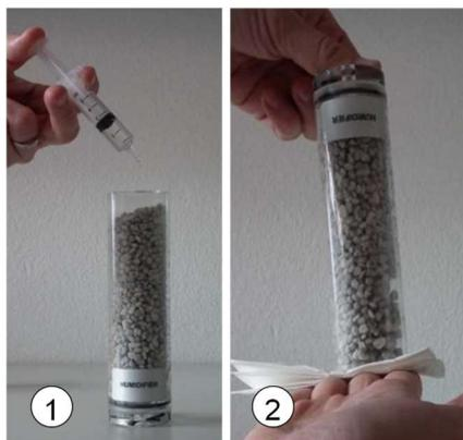
Ceramic granulate (Stuttgarter Masse) is used for humidifying the air. It must be wetted with distilled water. Please ensure that no water accumulates at the bottom of the tube. To prevent this, add the water slowly (1) so that it can be absorbed by the granulate. Carefully shake out excessive water before connection (2). The ceramic granulate can be autoclaved to prevent algae growth. The humidifier
