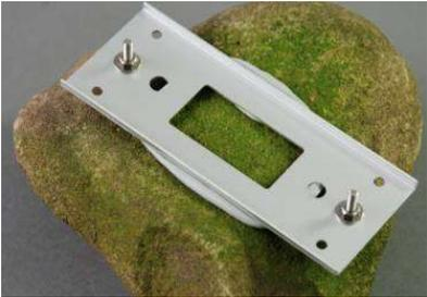
Use a surface-sealing plate for the air-tight connection to the sample. Make sure to model a defined area with Terostat IX® (Teroson, Henkel) with no dark gaps.
