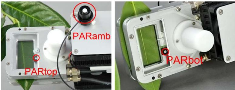
Fig. 22: Standard Measuring Head 3010-S, location of PAR sensors.
