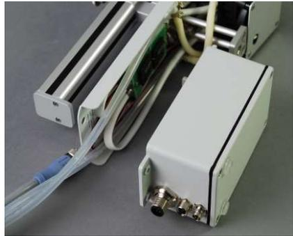
Disconnect the cable and remove the external light sensor. Remove the four screws holding the electronics box in place. Remove the electronics box from the measuring head as described in chapter 13.8.6. To not proceed without reading this chapter, because the electronics and the pins may become destroyed, if no care is taken.
