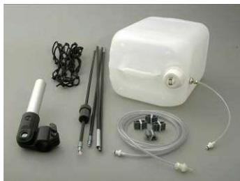
consisting of 10 l mixing vessel, 2.5 m fiberglass antenna, tubing with entrance filter, clips, elastic net and antenna holder for running the GFS-3000 in the field, using ambient air.
