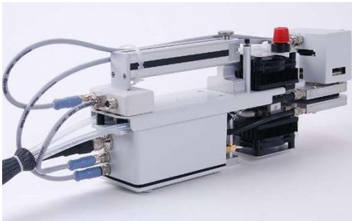
The adapter 3050-F/A extends the number of connectors of the measuring head. It is required, when using the Fiberoptics /PAM-Fluorometer 3050-F together with the Light Source 3041-L. Insert the adapter under the handle and
