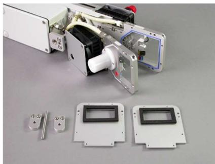
For thorough cleaning of the measuring head, the adapter plates should be removed, and the cuvette halves should be detached from each other for better access. (Do not! unscrew any screw of the external heat exchangers, also avoid any stress on the external heat exchangers).
