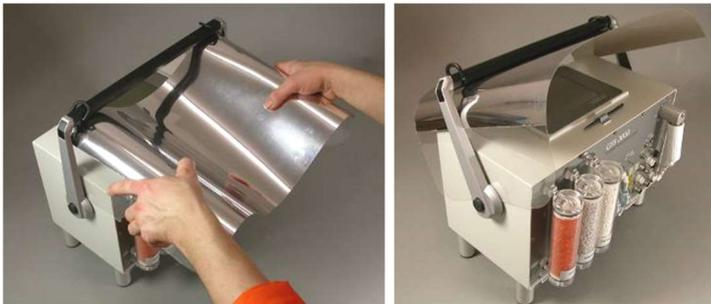
A sun screen can be installed underneath the handle of the control unit in the indicated way.
