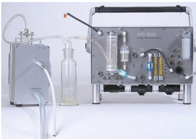
Fig. 62: Connection of the humidifier bottle. Water bubbles, when the pump will be switched on. Outlet of cold trap must be disconnected.
