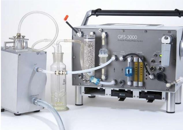
Fig. 63: Final set-up for H<sub>2</sub>O span calibration .
