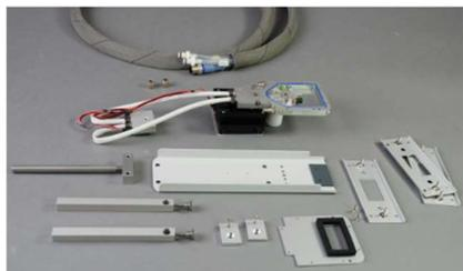
Screw the flat adapter plate to the lower cuvette frame and connect the tubing without any branch connections. Connect the tube labeled "To" to inlet #3 and the tube labeled "From" to outlet #4.
