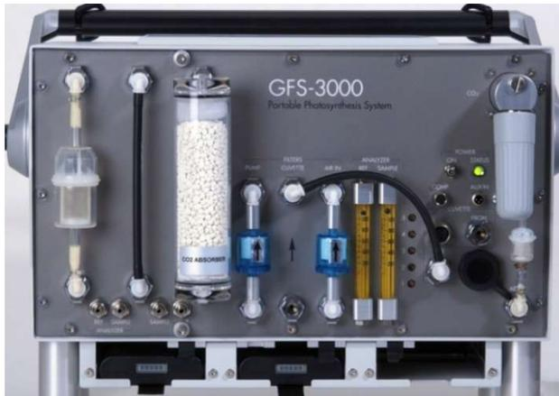
Fig. 58: Set-up of the system for CO<sub>2</sub> absolute zero calibration.
