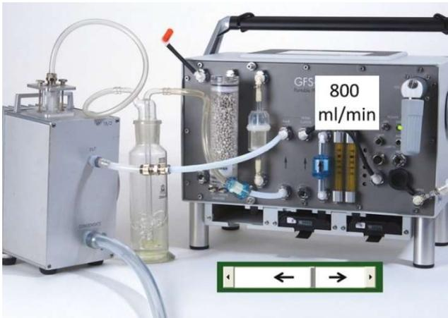
Fig. 64: Set-up for H<sub>2</sub>O span and software sliding bar.
