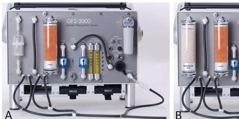
Fig. 60: Set-up for H<sub>2</sub>O zero calibration with air-cycling, A: First dry with Silica gel, B: Additionally, use MOLECULAR SIEVE for drying.
