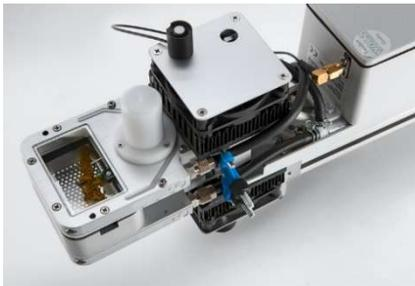
As an alternative to the cylindrical chamber, a rectangular chamber can be used for lichens or mosses. It consists of half a conifer chamber at the upper side and a flat adapter plate on the lower side. This set-up includes shorter spacers for the hinges and a shorter rod for the closing mechanism than the conifer chamber.
