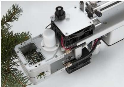
To replace the standard leaf area adapters with the conifer cuvette, it is necessary to increase the distance between the two cuvette frames. The hinge of the lower frame is mounted to the upper frame with two spacers.
