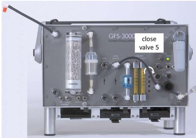
Fig. 61: Set-up of the GFS-3000 for H<sub>2</sub>O span calibration with GFS-Win version 3.31 or higher.
