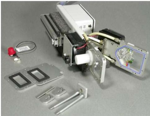
In the setup for the *Arabidopsis* chamber, the measuring head is laid on its side. The bottom side is detached, so that it can be turned upwards and connected to an angled adapter with opening for a pot holder.
