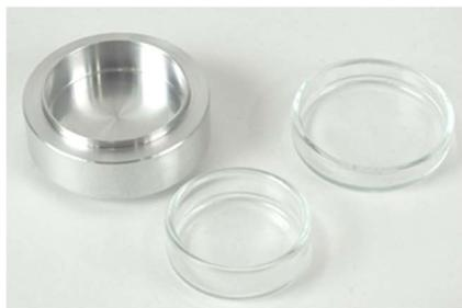
The cuvette for Petri dishes fits the Schott Petri dish (article number at Schott: 237553903, outer diameter of lid: 40 mm height: 12 mm). In this setup the measuring head is turned upside down and fixed with the handle-tripod adapter to the tripod as described in the chapter above. The setup has a closed plate underneath the aluminum block and a round adapter plate with opening at the upper side.
