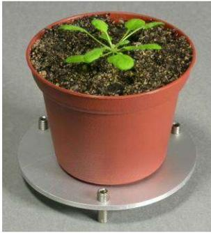
Lay the base plate into the lower part of the pot holder and place the pot in the middle of it. The adapter plate has the right elevation when the applied but not fixed top of the pot holder shows a gap of about 1 mm to the bottom part. Only in this configuration the upper brim of the flower pot is sealing completely with the foam in the upper part of the pot holder. Now a plant can be inserted into the chamber:
