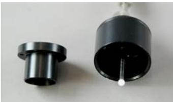
The adjustable black hood for suspension cuvettes has two configurations: with or without inner ring. With inner ring, it fits the Emitter-Detector Unit PHYTO-ED for round cuvettes.
