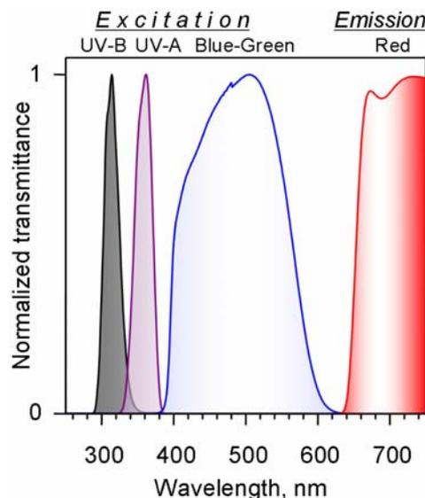
Fig. 1. Normalized transmittance of excitation and emission filters used to determine *in vivo* epidermal transmittance.
