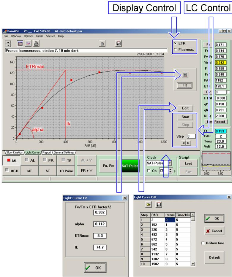
Fig. 17: Light Curve Window. In the present version of the software, below the **Fit** button, either the EP (Eilers an Peeters fit model) or the Platt et al. fit model can be selected.
