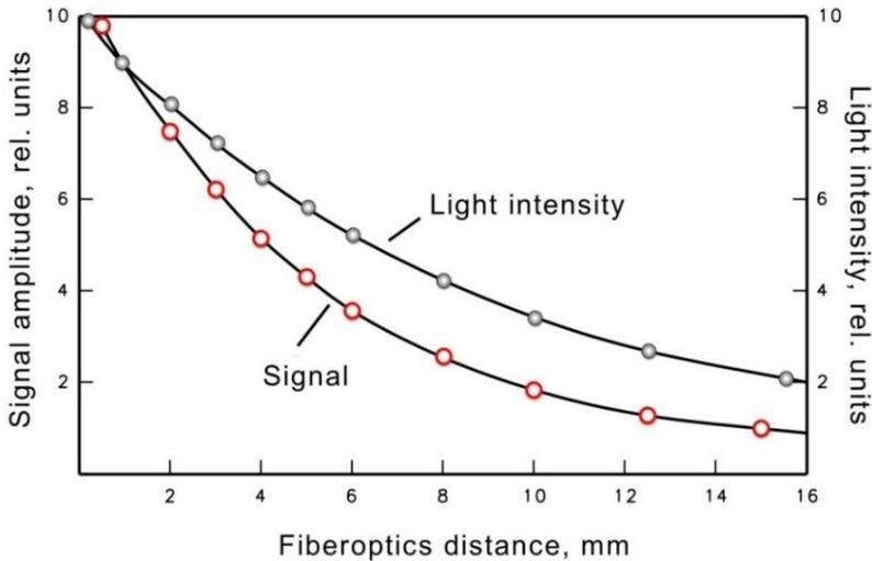
Fig. 4: Relationship between signal amplitude/light intensity and distance between fiberoptics exit plane and sample
