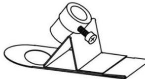
**Fig. 3: Distance Clip (to position leaf with respect to fiberoptics)**
