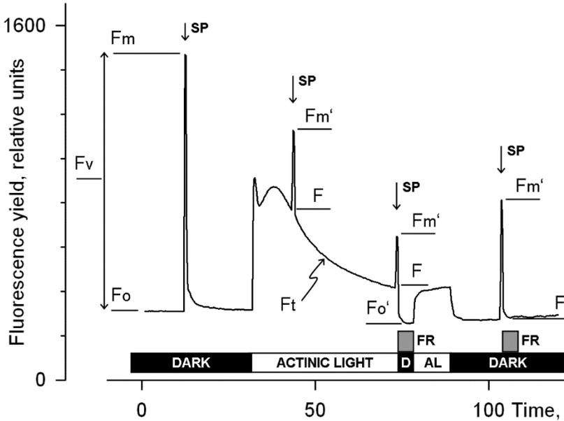
Fig. 25: Measurements for Saturation Pulse Analysis. AL, Actinic Light; D, dark; SP, Saturation Pulse; FR, far-red illumination.
