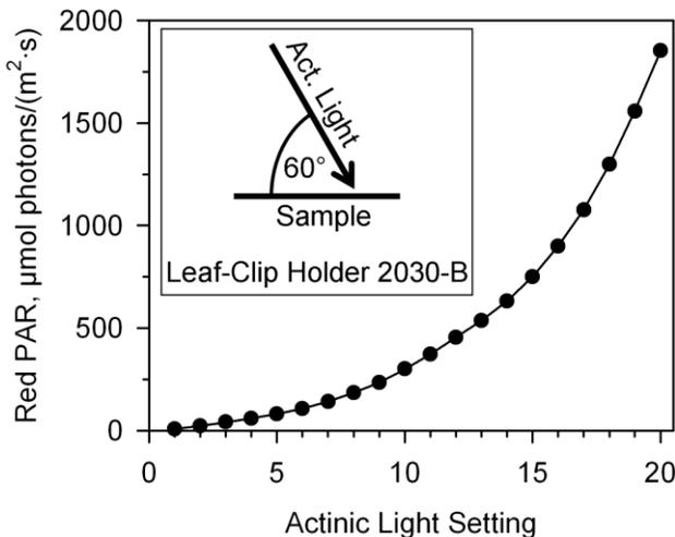
**Fig. 14:** Red Actinic Light Intensities at Sample Level of a Leaf-Clip Holder 2030-B.
