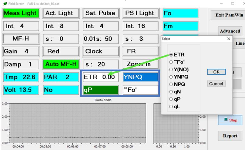
Fig. 11: Field Screen. The blue square surrounds the four fields for the selectable parameters. On clicking on one of these four fields a menu pops up that allows the selection of a parameter for this field.
