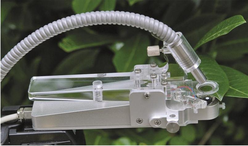
**Fig. 5: Leaf-Clip Holder 2030-B with Fiberoptics 2010- F.**
