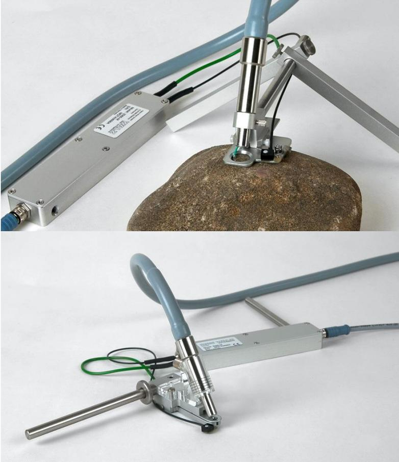
**Fig. 6: Fiberoptics holder for Surfaces 2060-A (top) and Arabidopsis Leaf Clip 2060 (bottom) in combination with the mini-quantum/temp. sensor 2060-M.**
