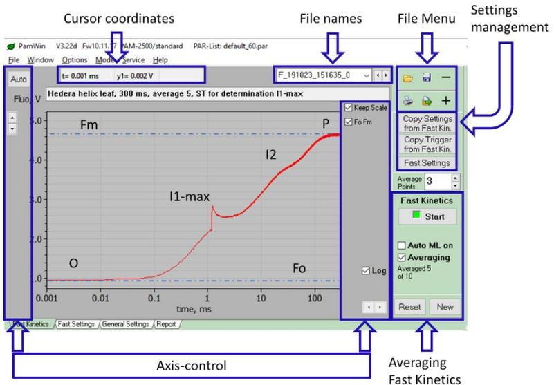
Fig. 21: Fast Kinetics Window. For the transient shown in the figure, 5 measurements (spaced 4-5 min apart) were averaged. A 50  $\mu$ S ST was applied after 2 ms of illumination for the determination of the I1-max level.
