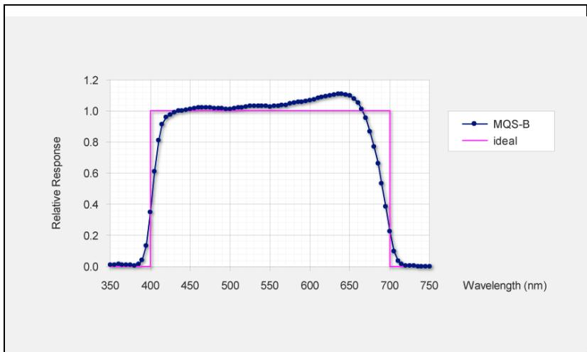
**Fig. 4: Spectral response of MQS-B sensor**
