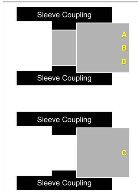
**Fig. 2: Positioning of fiberoptics adapters in sleeve coupling of MQS-B/A adapter set.**
