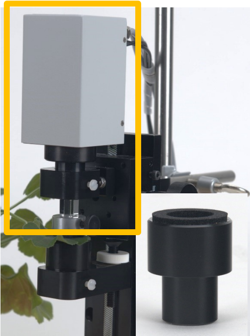
Fig. 8: the stand-alone configuration of the MCP-II-EDST (strong flash lamp) unit of the MULTI-COLOR-PAM-II for flash measurements on leaves. The bottom unit (also see the inset) is there to keep the leaf in place.
