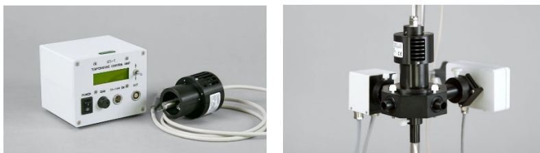
Fig. 11: US-T Temperature Control Unit. Left, the heat-transfer head with the Peltier element and the Control Unit; right, the connection between the head and the ED-101US/MD optical unit.
