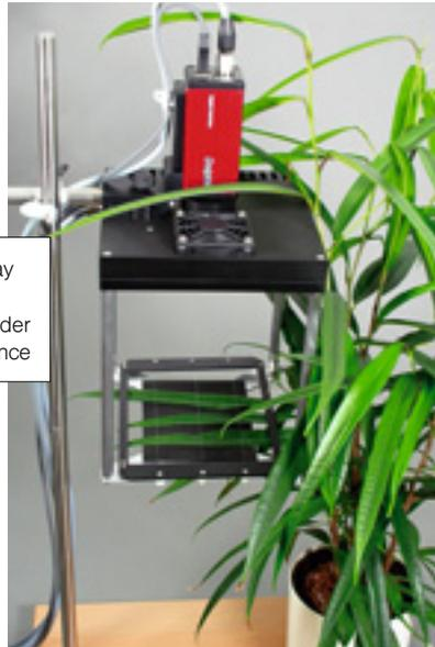
Measuring Head (LED-Array plus camera) mounted on separate stand with leaf holder providing fixed working distance
