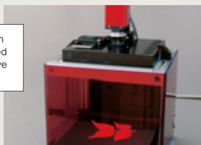
Standard configuration with LED-Array and camera fixed on Mounting Stand with Eye Protection
