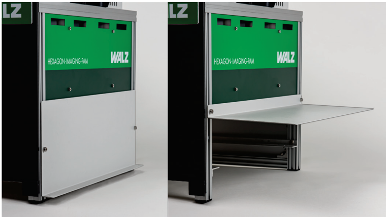
Fig. 7 Use of the supplied screens to protect the user from reflections. On the left side the instrument is completely closed and can be used with the base plate in the highest position or without the baseplate for potted plants. On the right side the user is still protected from direct glare but plant trays can still be inserted from the side.
