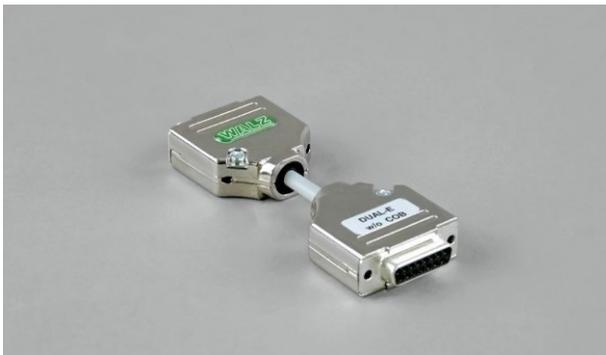
Fig. 13: Two-way Adapter for Unilateral Actinic Illumination DUAL-TW
