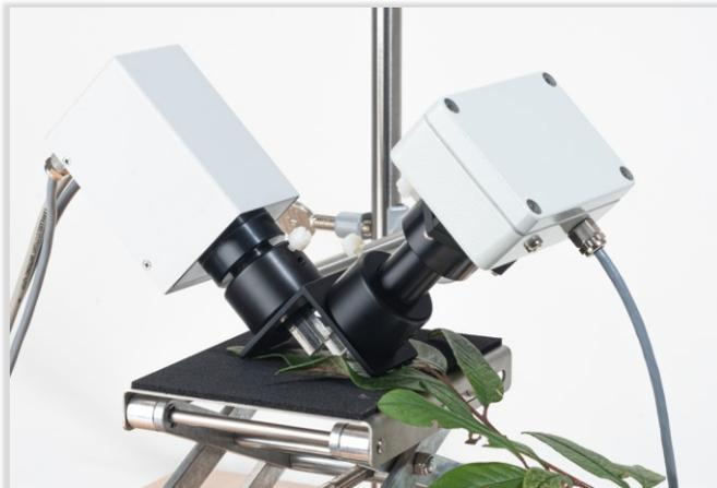
Fig. 10: 90 Degree Measuring Head Holder DUAL-H90
