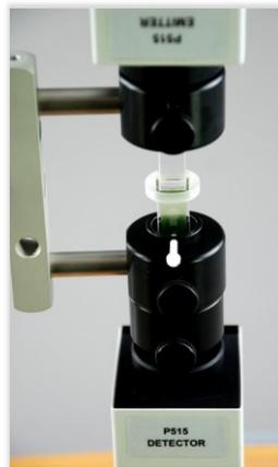
Fig. 22: Low-Drift Cuvette DUAL-K25
