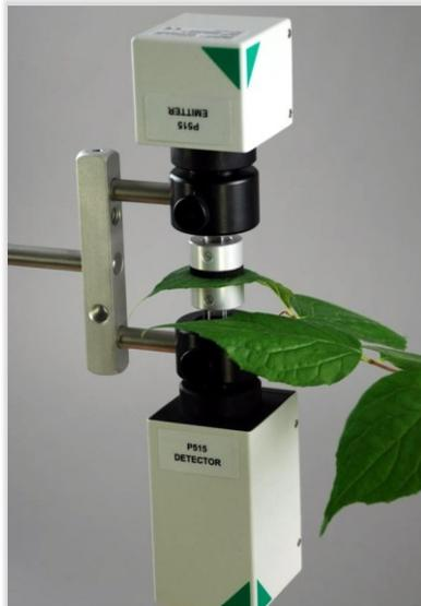
Fig. 14: P515/535 Emitter-detector Module
