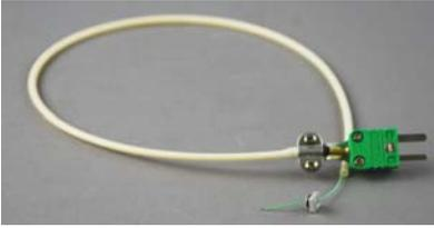
First switch power off. The thermocouple for measuring the leaf temperature is mounted in the lower cuvette frame.
