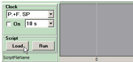
Fig. 23 Script buttons in lower right corner of Dual-PAM program user surface
