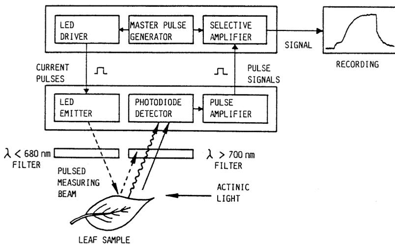
Fig. 16: Schematic view of the PAM measuring principle
