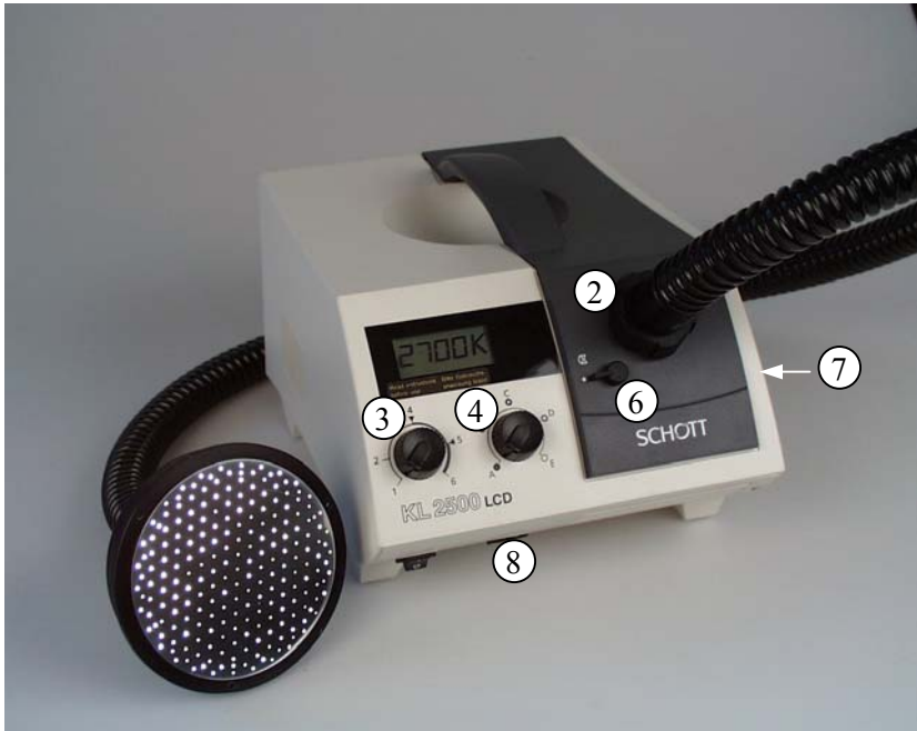
Fig. 1: Fiber Illuminator FL-460 with Special Fiberoptics 460-F (2: light guide connection; 3: electronic adjustment; 4: mechanical aperture; 6: supplementary optics; 7: filter wheel; 8: connection socket for remote operation; the numbers agree with those in the original manual)
