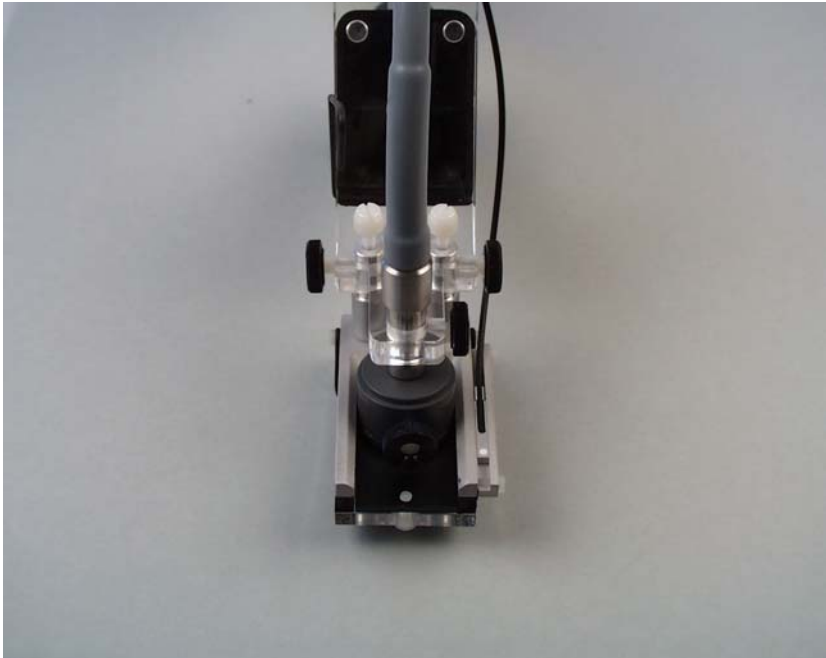
Fig. 5: 90° measuring geometry featuring Darkening Adapter and Darkening Plate installed in the lower "jaw"
