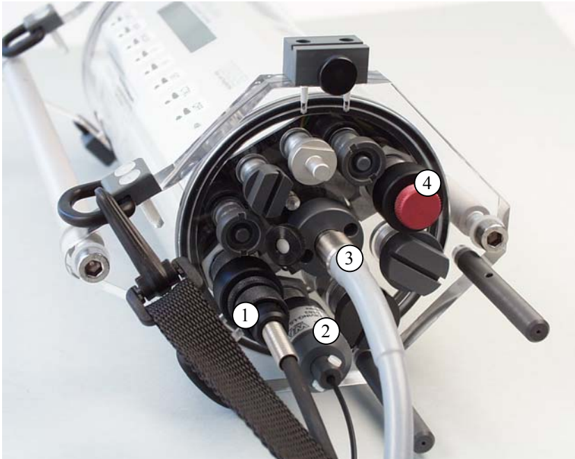
Fig. 2: Various connectors at the right hand side of the DIVING-PAM housing:
