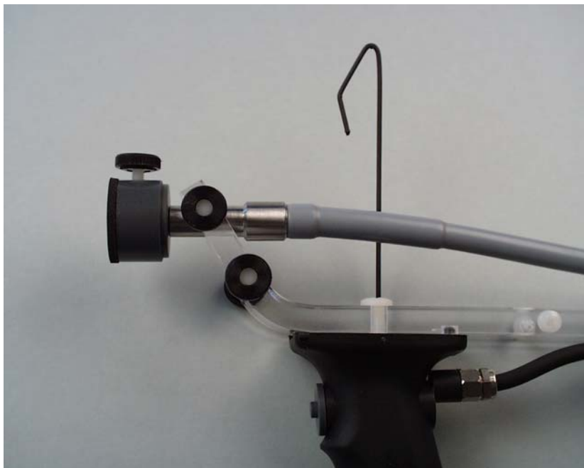
Fig. 7: Darkening Adapter in 90° geometry
