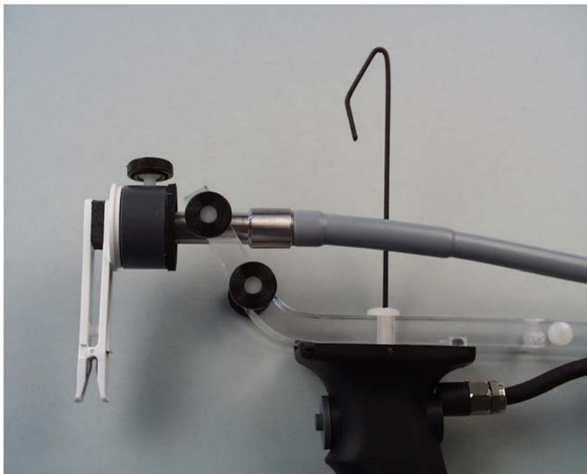
Fig. 9: Dark Leaf Clip DIVING-LC (optional accessory) connected via the back side of the Darkening Adapter to the Fiberoptics
