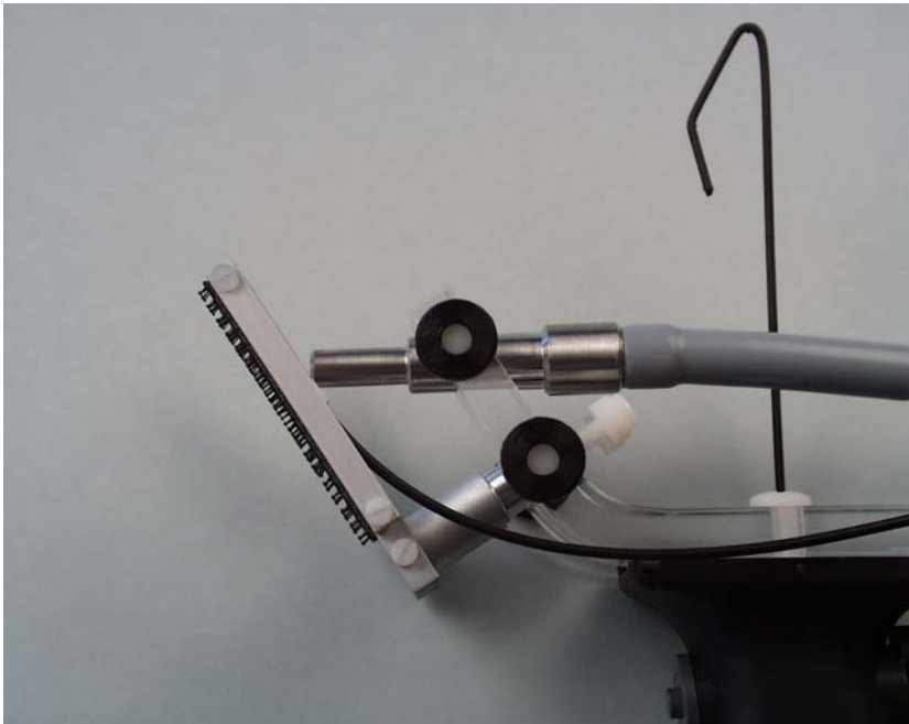
Fig. 6: 60° geometry with lower jaw being removed
