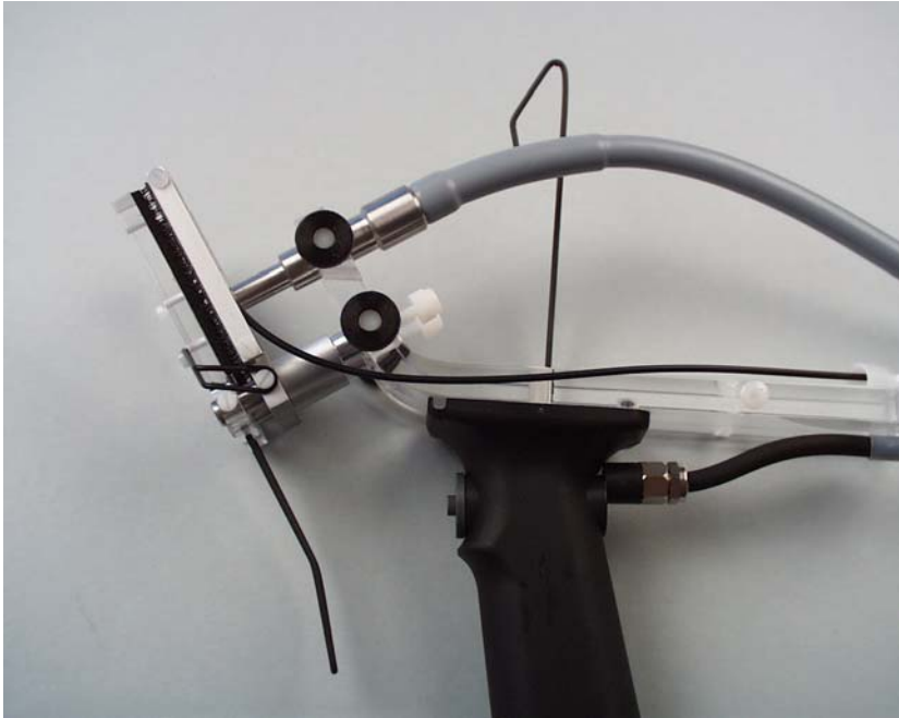
Fig. 4: 90° measuring geometry recommended for recordings of Light- and Induction-Curves
